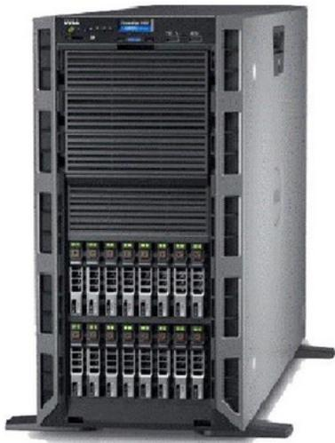
*Intel Xeon E5-2630 v3 (20M Cache, 2.40 GHz), 16GB DDR4 2133MHz, 16 x 2.5" SAS/SATA, PERC H730 1GB, DVD-RW, Matrox G200 16MB, Gigabit Ethernet, iDRAC8 Express, 750W*
